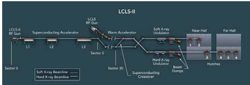
Figure C.1.2: FELs are linear accelerators, consisting of the injector, a cathode in a strong field RF cavity, from which electrons are emitted upon illumination with a short laser pulse, an accelerator section (L1-L3) with bunch compression and a cascade of undulators, in which the coherent radiation is generated. The image shows the layout of LCLS-I, which has Cu accelerators, labeled (Warm Accelerator) and LCLS-II, which will feature superconducting cavities for acceleration that can be operated in CW mode. The pictures are taken from the LCLS-II website with permission from LCLS.
